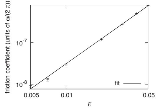
FIG. 8. Linear damping of the horizontal momentum in systems without horizontal restitution as a function of the coupling  $E$ . Note that the time-scale separation parameter  $\epsilon$  equals the slope  $E$ . Apart from  $E$ , all parameters are as in Fig. 7. The fit corresponds to a second-order dependence on  $E$ .
