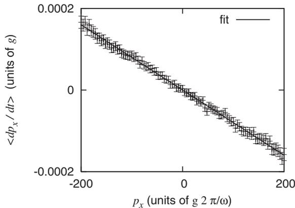
FIG. 7. Average drift in the horizontal momentum as a function of the horizontal momentum in a system without horizontal restitution. Parameters:  $E=0.05$ ,  $4\pi^2g/(\omega^2A)=0.2083$ ,  $\alpha=1$ , and  $\beta=0.9$ .
