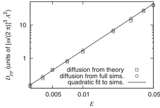
FIG. 6.  $D_{pp}$  as a function of  $E$  for  $p_x=0.0$ ,  $4\pi^2g/(\omega^2A)=0.2083$ ,  $\alpha=1$ , and  $\beta=0.5$ . The fit is quadratic and shows that the numerical results are consistent with the theory, Eq. (23).
