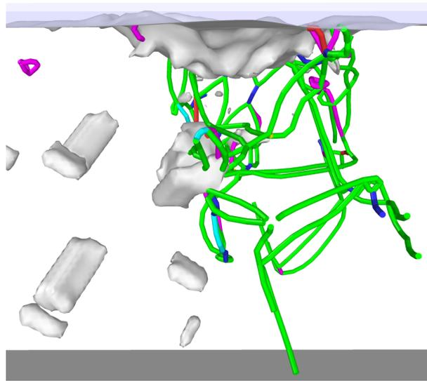
Figure 3: Molecular dynamics simulation of a nanoindentation of aluminium including particles. The lines visualize the dislocations and the blobs are Mg-Si particles.
