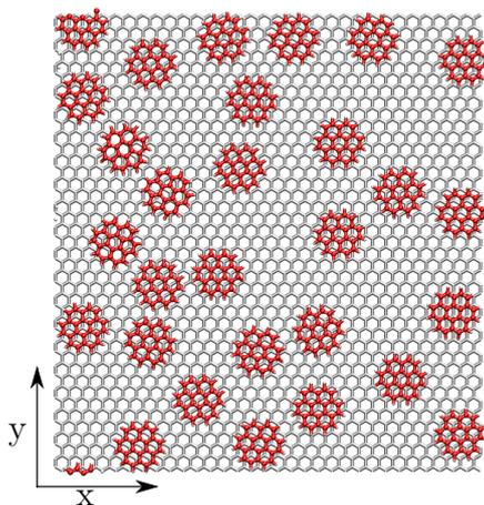
Figure 2: A top view of a simulation of a single layer of graphene flakes acting as a solid lubricant.
